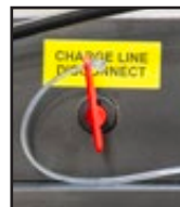
Charge Line Disconnect (red key)
