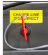
Charge Line Disconnect (red key)
