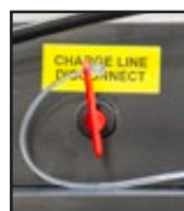
Charge Line Disconnect (red key)
