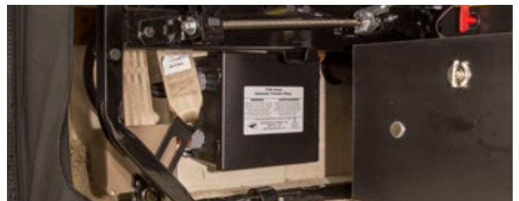
ARM DOWN INDICATES TRIPPED BREAKER
