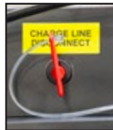
Charge Line Disconnect (red key)
