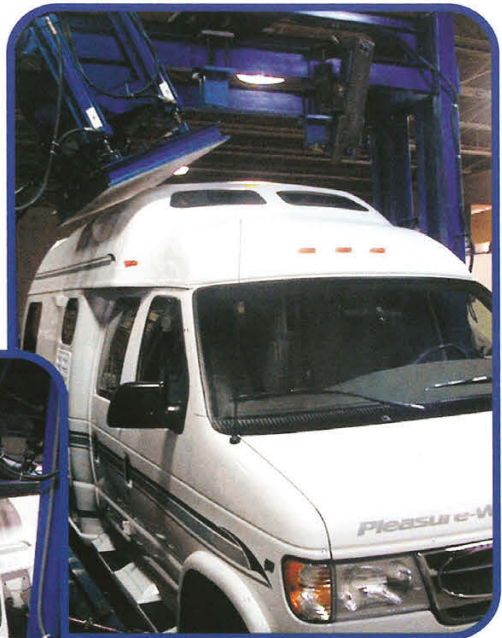
Roof Crush Resistance Testing
