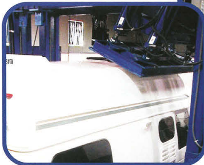
Roof Crush Resistance Testing
